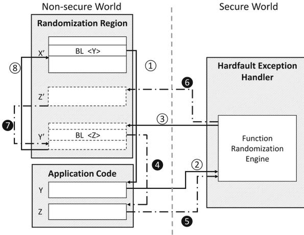
**Fig. 2.** Program flow of function *X*, *Y* and *Z*. For any function *F* in the NS app, we use *F'* to represent its corresponding copy in the randomization region.
