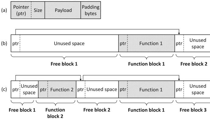
**Fig. 3.** Memory management. (a) Structure of the randomization region; (b) Memory layout before loading Function 2; (c) Memory layout after loading and randomizing Function 2
