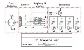
Fig. 3. Schematic of the IR transceiver board.
