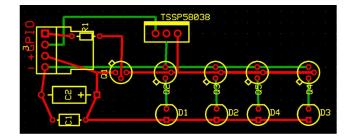
Fig. 4. PCB design of the IR transceiver board.
