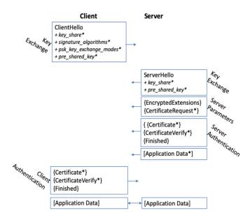
Fig. 10. TLS 1.3 handshake. + refers to extensions in a message; \* refers to optional or situation-dependent messages/extensions; {} refers to messages encrypted using keys derived during handshake; [] refers to messages protected using keys derived through handshake [29].
