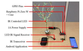
Fig. 6. IR device setup.
