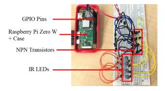
Fig. 8. LED radiation intensity test setup.
