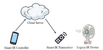
Fig. 2. System architecture.
