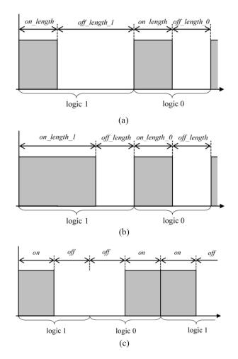
Fig. 1. IR signal encoding. (a) Pulse distance. (b) Pulse length. (c) Bi-phase.
